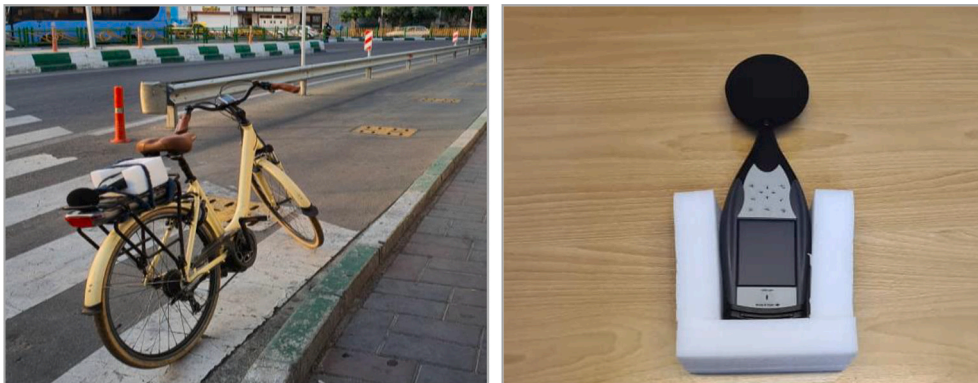
Fig. 4. Portable sound level meter, B&k 2250 model.
