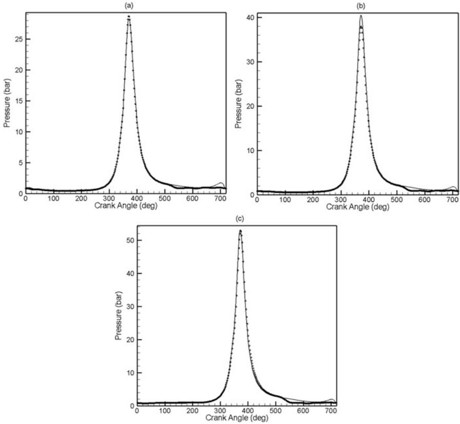
**Fig. 12** In-cylinder pressure profile for fuel 3 at compression ratio of 16 for (a) BMEP = 2 bar, (b) BMEP = 4 bar and (c) full load conditions. Solid lines denote simulation and symbols denote experimental results
