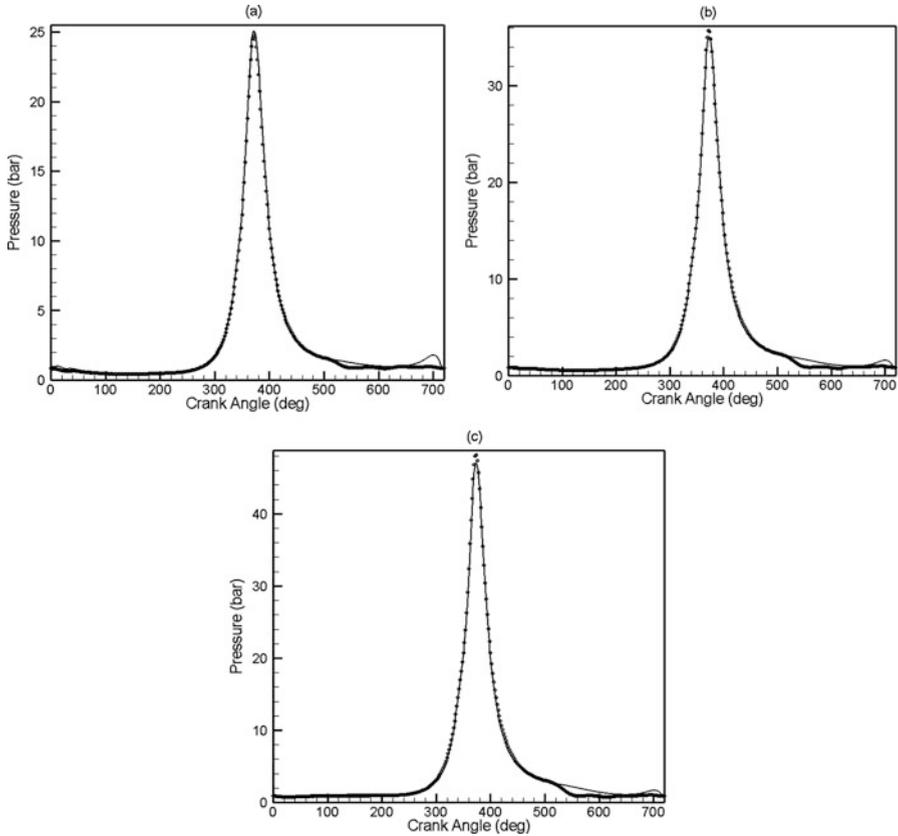
**Fig. 7** In-cylinder pressure profile for fuel 1 at compression ratio of 14 for (a) BMEP = 2 bar, (b) BMEP = 4 bar and (c) full load conditions. Solid lines denote simulation and symbols denote experimental results
