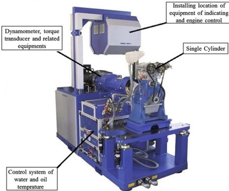
**Fig. 1** Illustration of the test bed (Javaheri et al. 2014)
