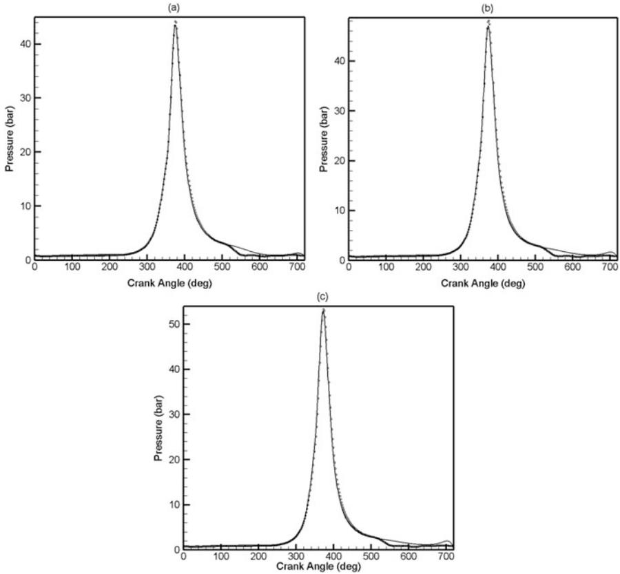
**Fig. 9** In-cylinder pressure profile for fuel 2 at (a) CR = 12 bar, (b) CR = 14 bar and (c) CR = 16. Solid lines denote simulation and symbols denote experimental results
