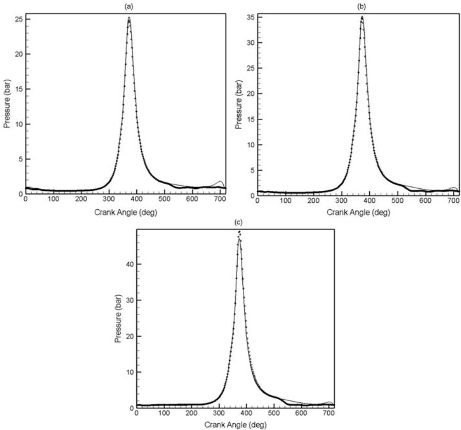
**Fig. 11** In-cylinder pressure profile for fuel 3 at compression ratio of 14 for (a) BMEP = 2 bar, (b) BMEP = 4 bar and (c) full load conditions. Solid lines denote simulation and symbols denote experimental results
