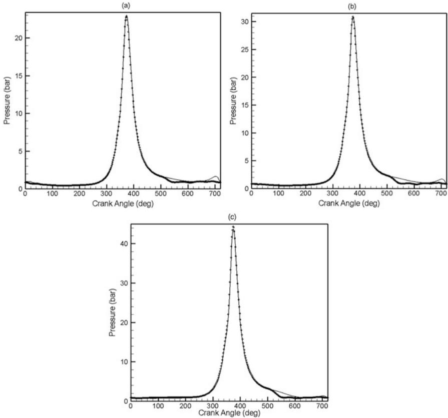
**Fig. 6** In-cylinder pressure profile for fuel 1 at compression ratio of 12 for (a) BMEP = 2 bar, (b) BMEP = 4 bar and (c) full load conditions. Solid lines denote simulation and symbols denote experimental results
