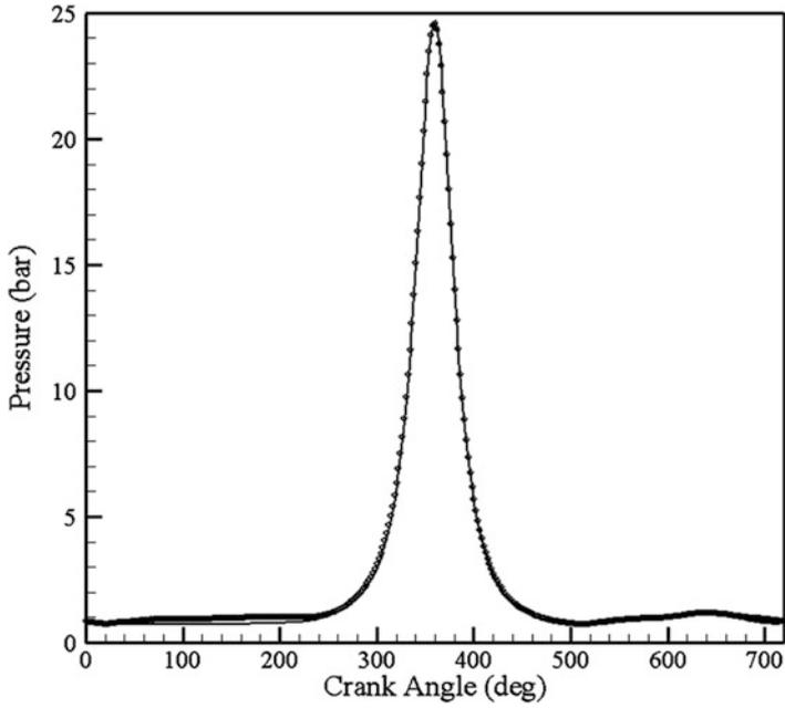
Fig. 4 In-cylinder pressure profile for motoring condition at CR = 14
