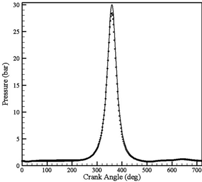
Fig. 5 In-cylinder pressure profile for motoring condition at CR = 16
