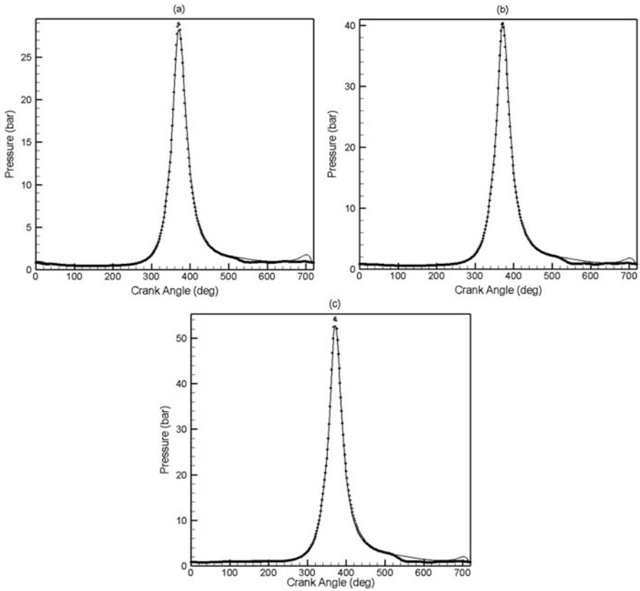
**Fig. 8** In-cylinder pressure profile for fuel 1 at compression ratio of 16 for (a) BMEP = 2 bar, (b) BMEP = 4 bar and (c) full load conditions. Solid lines denote simulation and symbols denote experimental results
