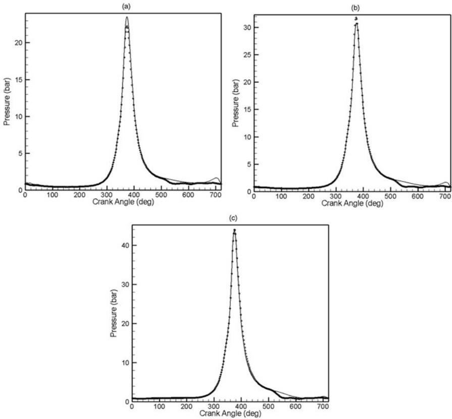
**Fig. 10** In-cylinder pressure profile for fuel 3 at compression ratio of 12 for (a) BMEP = 2 bar, (b) BMEP = 4 bar and (c) full load conditions. Solid lines denote simulation and symbols denote experimental results
