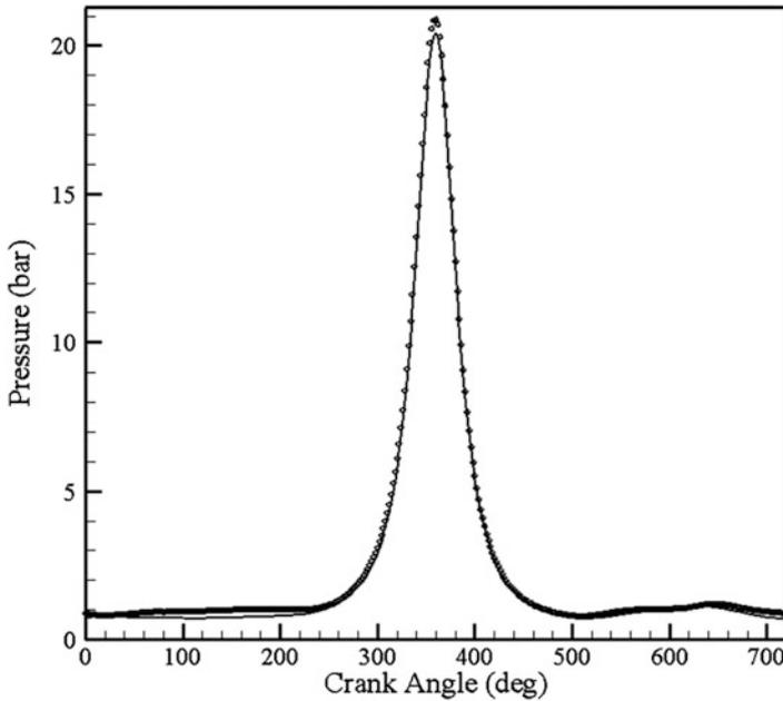
**Fig. 3** In-cylinder pressure profile for motoring condition at CR = 12
